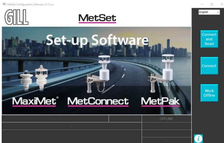
MetSet can be used to create a user specific set-up that can be loaded onto MetConnect.
