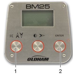
Figure 14: press 1 and 2 to select the calibration gas
