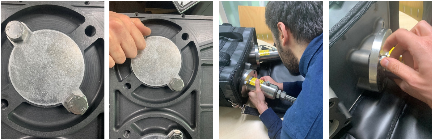
Figure 13. Demonstration of how to mount the transducers onto the Fluenta FlareCal™ box.
