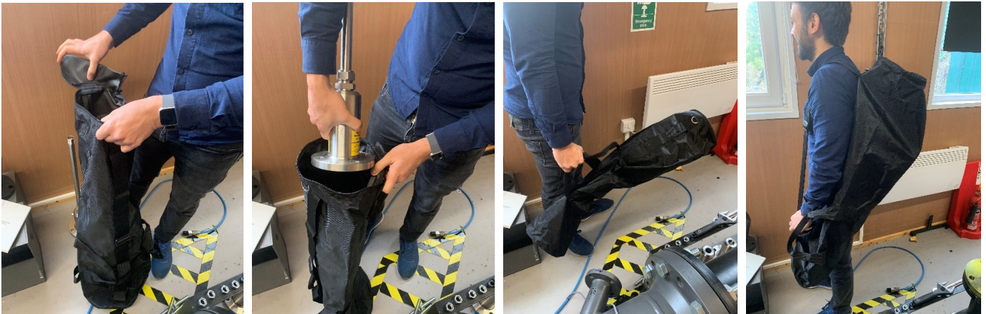
Figure 12. How to use the supplied transducer carry bags to transport transducers safely.
