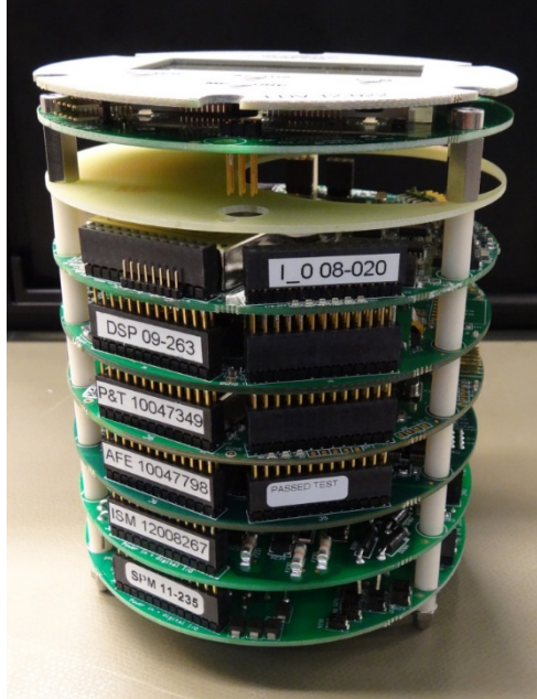
Figure 4: FGM 160 flow computer electronic modules.
