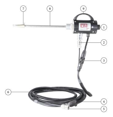
► Check the probe filter before and after each measurement.
