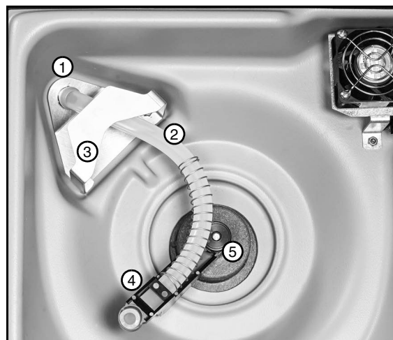
Figure 2-2 Attaching the distributor arm and discharge tube
