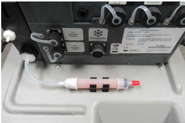
Figure 2-21 Desiccant cartridge installed into the side retaining clips.
